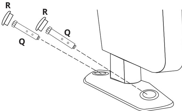
Use the **Concrete Anchors (Q)** to secure the feet of the **Chair Legs** to the floor.
