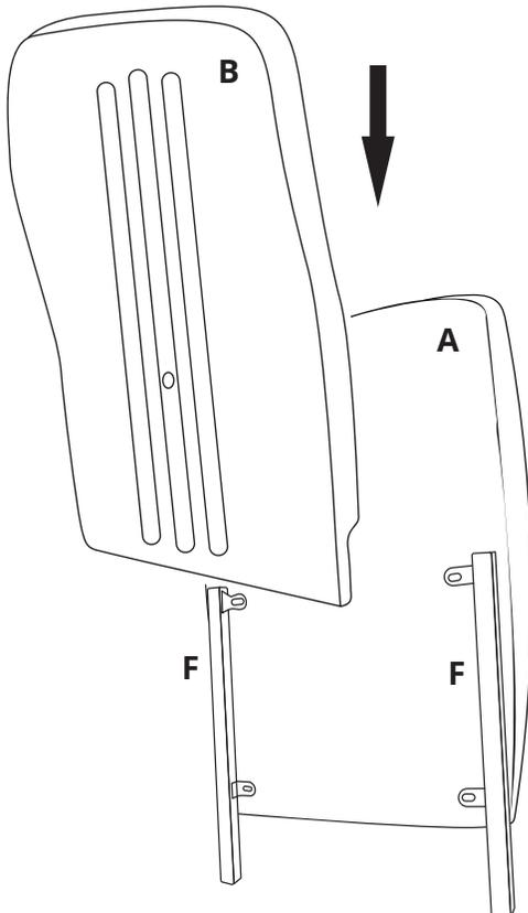
Slide the **Seat Back Shell (B)** on to the **Support Bars (F) x 2** with the **Seat Back Cushion (A)** attached.
