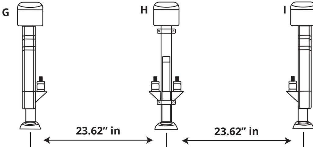
Place **Right Chair Leg (G)** into the desired placement (do not attach to floor). Measure 23.62" in (600mm) then place the **Middle Chair Leg (H)**. Measure 23.62" (600mm), then place **Left Chair Leg (I)**. Measurement is from centerline bolt to the next centerline bolt. Repeat for as many chairs as needed.
