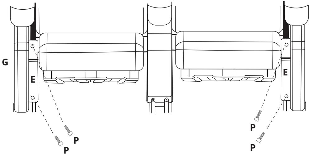
The **Trim (E)** is used on the outer **Left and Right Chair Legs (G) & (I)**. Attach the **Trim (E)** with **Hex Screws (P)** on the corresponding **Chair Legs**.
